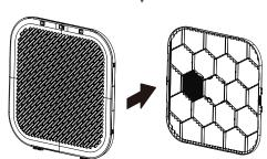
Separate the frame from the filter assembly.
